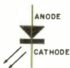
Fig. 1. Schematic symbol for LED is standard diode with arrows for light output.
