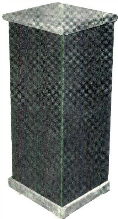
Grille cloth goes around body of enclosure. Bottom bumper must extend no lower than tops of enclosure's feet.
