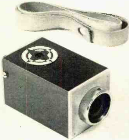
A compass, photocell, and Mallory Sonalert combine to produce electronic compass with audible output. Device uses a penlite cell.
