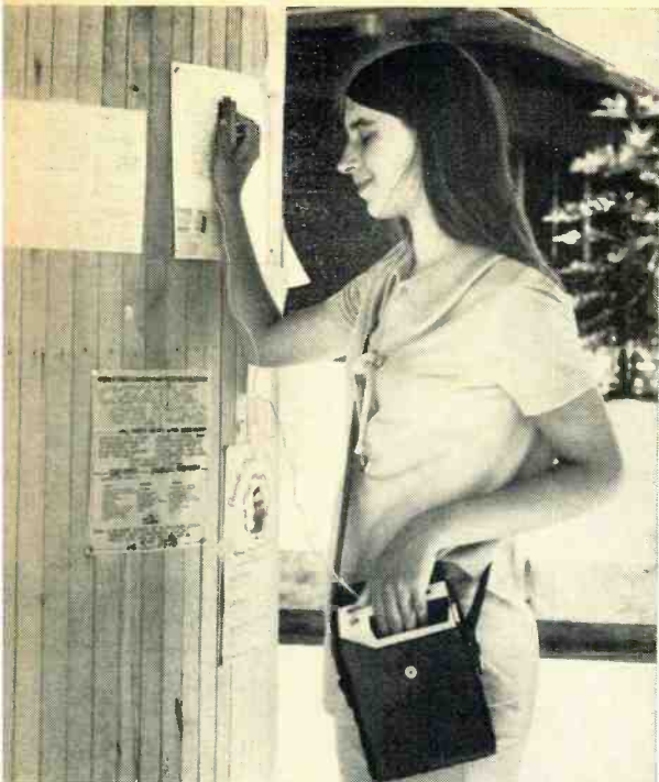
Shari Gabrielson, Berkeley High School student, reads bulletin board with an Optacon reading machine developed at Stanford Univ. While scanning with probe in right hand, her left hand makes contact with an array of tiny tactile stimulators which form outline of each scanned letter. Single finger tip can be employed to read the letters.
