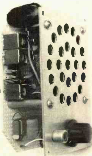
Photo shows how perforated board, with the components, is attached to the front panel.
