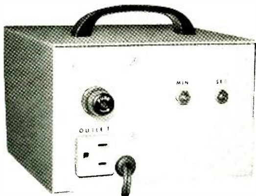
Mounted on the back panel are the power outlet, the fuse, and adjustments R2 and R3.
