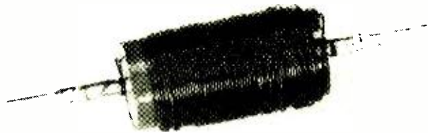
Fig. 6. A hand-wound shunt resistor. Next the assembly is protected with a coil dope.
