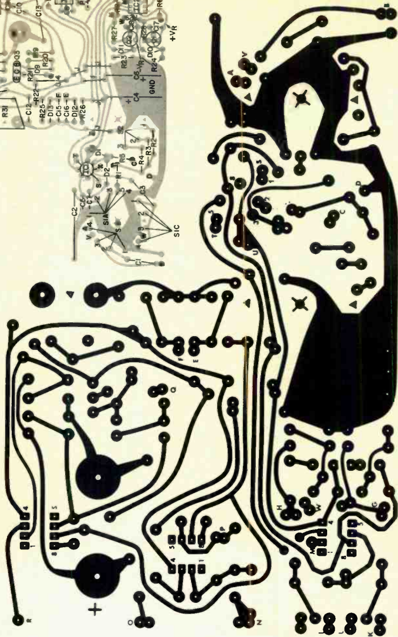
Fig. 3. Actual-size foil pattern for Super Op is below; component layout shown at left.
