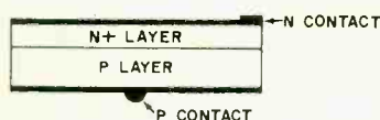
Fig. 1. Cross section of silicon solar cell shows its similarity to simple pn junction.
