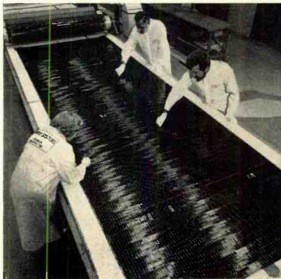
Fig. 8. Panel of solar cells for a Hughes FRUSA (Flexible Rolled-up Solar Array).
