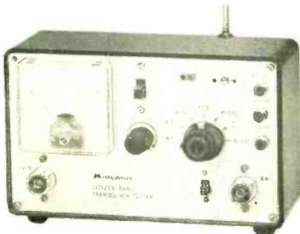
This CB test set by Midland checks anything from crystals to r-f output and efficiency.
