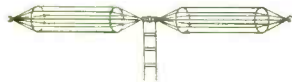
Fig. 2. Cage type of multi-wire dipole. Though a two-wire feeder is shown, this antenna can be adapted to conventional 52-ohm coaxial feedline.
