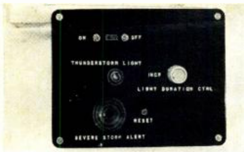
Front panel of Forecaster holds warning light and a severe storm alert.
