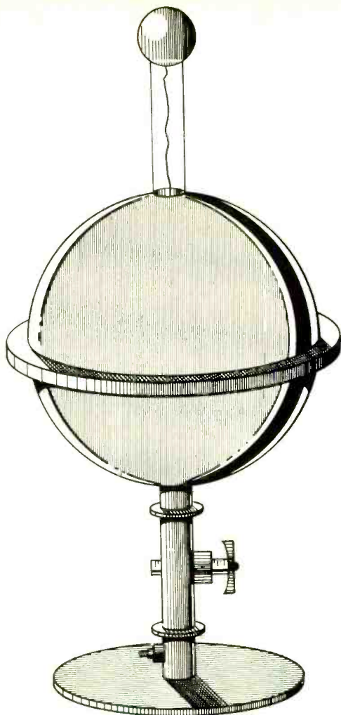
A Faraday Sphere. Faraday used this piece of equipment to determine the "specific inductive capacity" (which we now call the dielectric constant) of different types of insulating materials.
