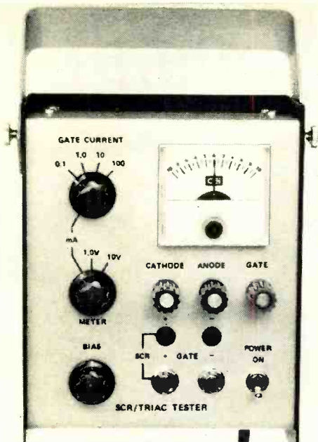
Front panel arrangement of prototype. LED's are mounted in rubber grommets.
