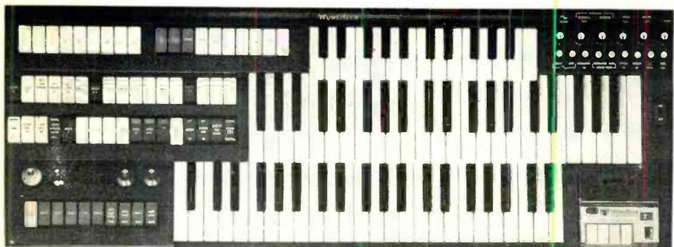
Fig. 1. The keyboard of the Wurlitzer 4037 organ, designed for the advanced amateur or the professional. Special modulator/attack keyboard is shown at upper right while the built-in cassette tape recorder is at the lower right.
