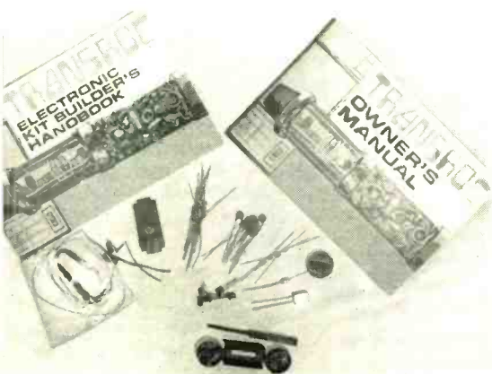
Several companies produce telemetry equipment for model rockets. Shown is Transroc, a kit operating on the Citizens Band with range of several miles paired with superhet receiver.
