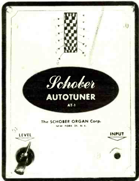
Fig. 6. Organ tuner has stroboscopic disc.
