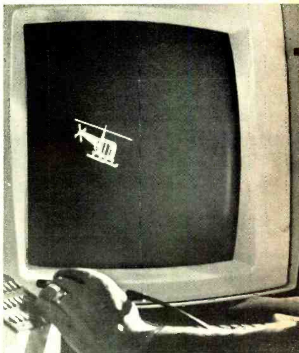
Prof. Charles Csuri, head of Ohio State U. computer art group, controls flight of helicopter drawn on a CRT.
