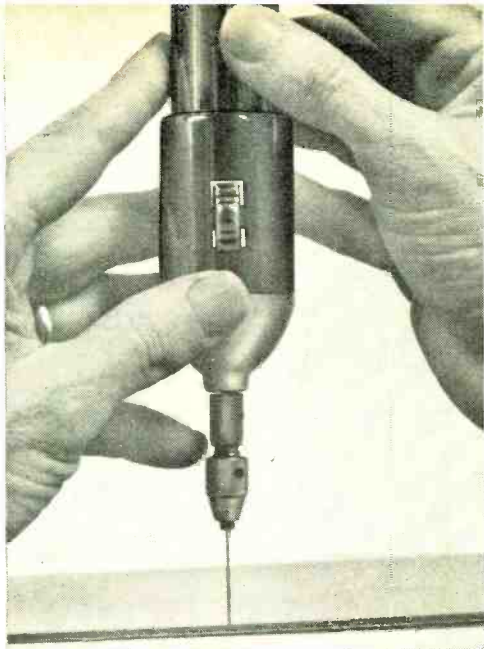
Fig. 1. To properly use battery-powered drill, when working on printed circuit boards, hold it perpendicular to work surface and apply minimal force.
