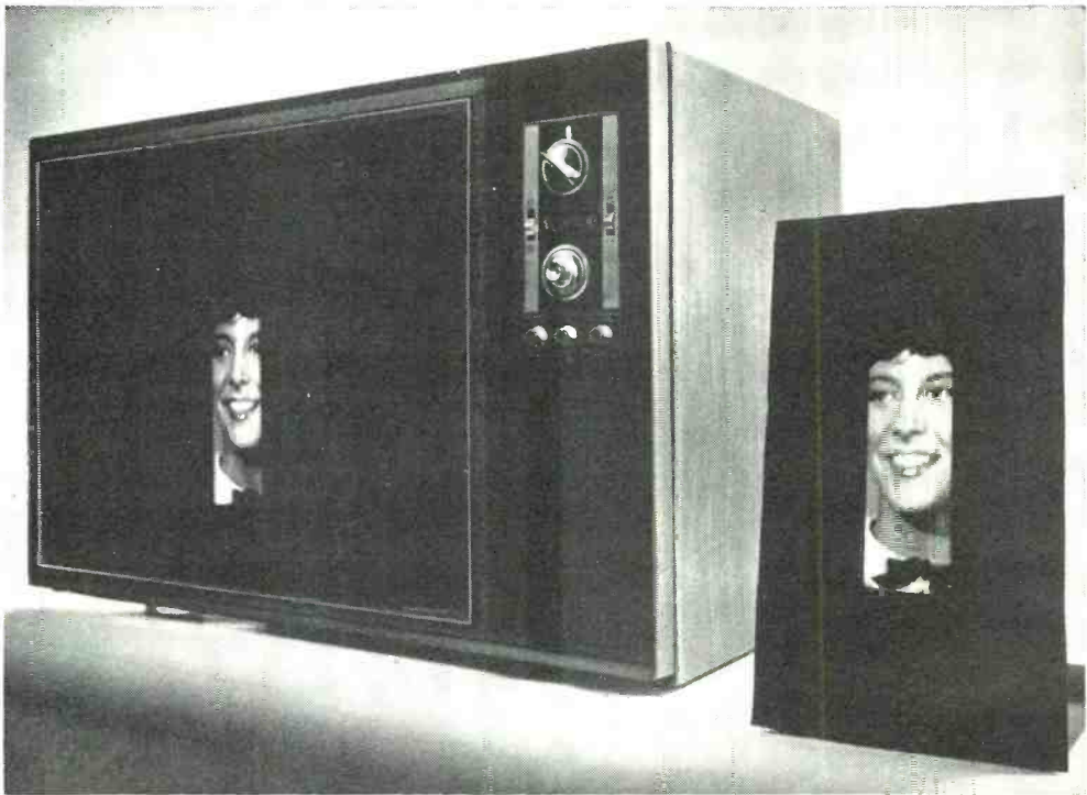
(Below) Without the associated electronics, the panel is only \frac{5}{8} " thick. (Above) Comparison between the thin panel and conventional color receiver. The receiver screen is masked to show same area as panel. (Right) Close-up of panel shows excellent resolution.
