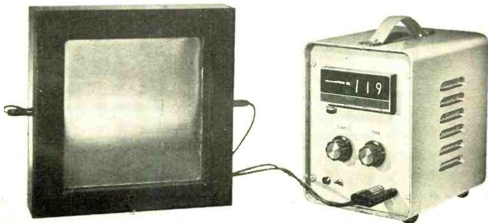
Fig. 1. Liquid crystal microwave power density meter made by Bendix.
