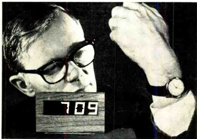
Fig. 2. Prototype liquid crystal digital readout for watches and calculators. (Photo: RCA Labs.)
