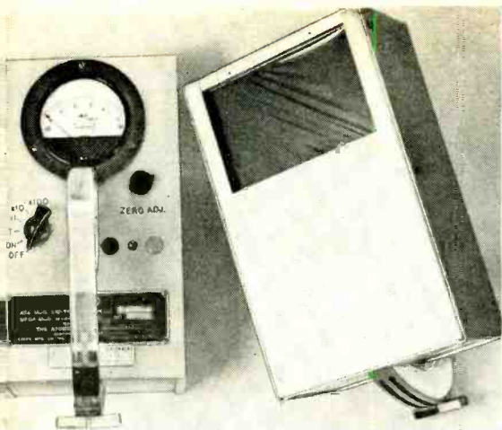
Fig. 2. Two views of ionization survey meter.
