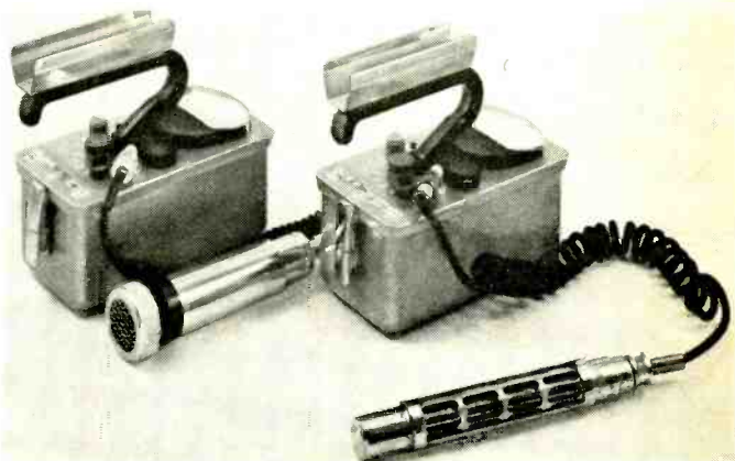
Fig. 8. (Left) End-window and (right) thin-wall Geiger-Muller survey meters.
