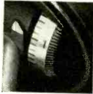
Stylus pressure dial calibrated in tenths of a gram from 0 to 1.5 grams; in quarters of a gram from 1.5 to 3.0 grams.
