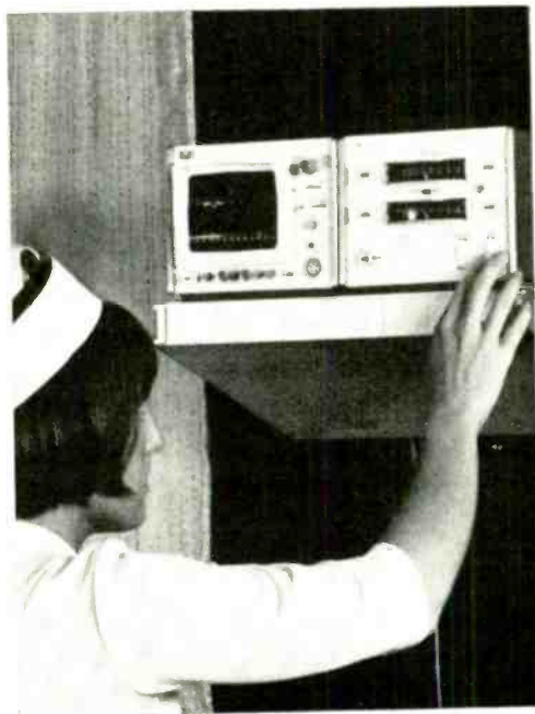
Bedside instruments monitor the patient's ECG, heart rate, and blood pressure. (Courtesy: Hewlett-Packard)
