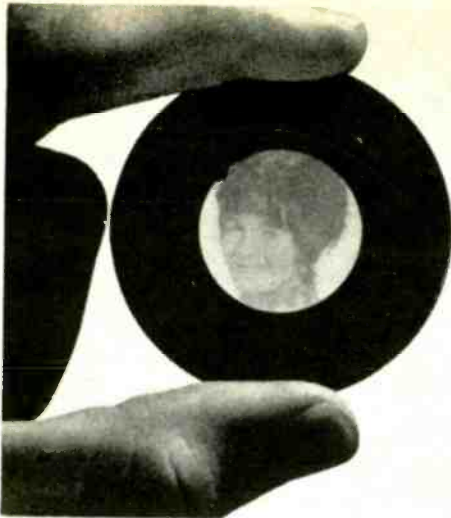
Positive image stored in a ceramic electro-optic device. Plate is 1 in. in diameter and is 0.0123 in. thick.
