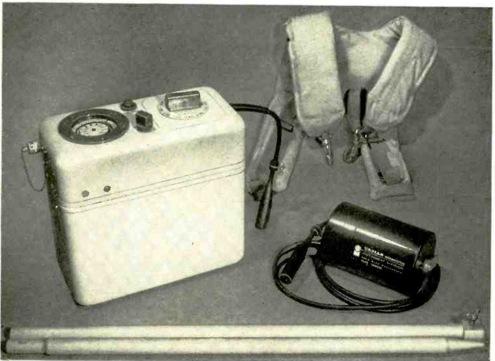
Fig. 1. Varian's proton free-precession magnetometer can be used on land; or, with the sensor head shown at right waterproofed, in an underwater environment.
