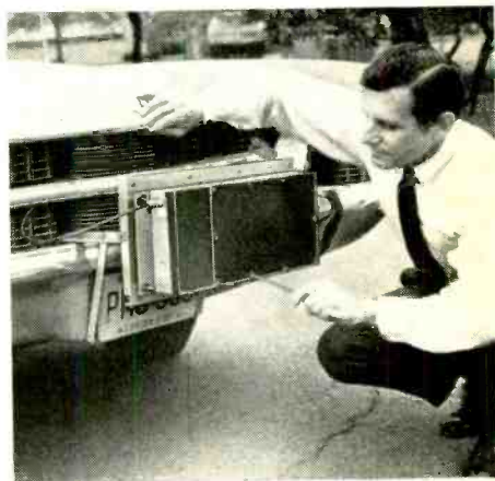
Radar transmitter is mounted on front bumper or behind grille or license.
