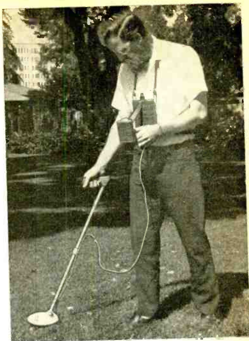
Fig. 2. In Fisher Explorer II, the electronics is carried by strap suspended around the prospector's neck.
