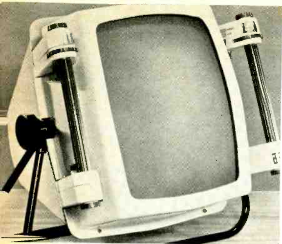
Plessey's unique MR-12 indicator has its operating controls in the handles.
