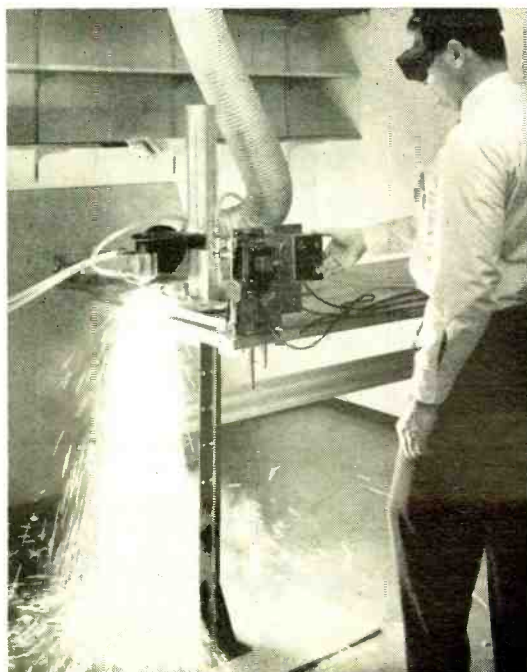
Above, quartz tubing is cut with Sylvania carbon dioxide laser. Below, jet of oxygen is used on Coherent Radiation laser to supply extra power for cutting titanium sheet.
