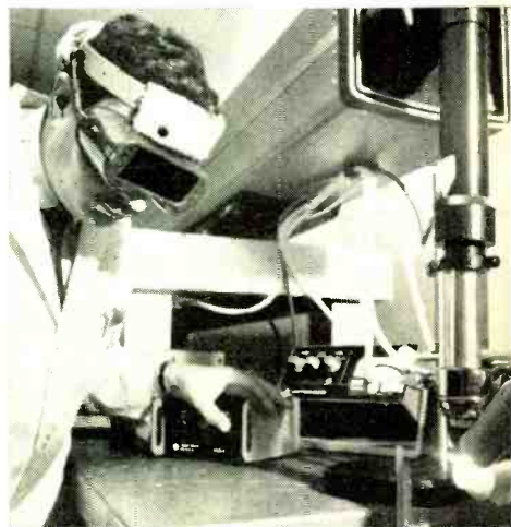
Above, quartz tubing is cut with Sylvania carbon dioxide laser. Below, jet of oxygen is used on Coherent Radiation laser to supply extra power for cutting titanium sheet.
