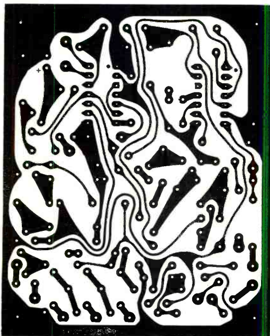
Fig. 5. Actual size drilling and etching guide and component placement and orientation diagram are shown left and below, respectively.
