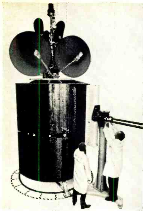
Intelsat IV satellite is shown here being tested in Hughes r-f laboratory.
