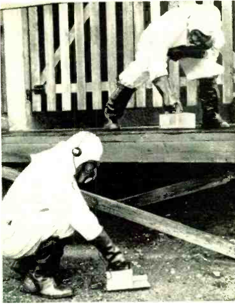
Emergency radiation team members at AEC's Hanford Works show how Geiger and scintillation counters are used to measure radioactive contamination should it get out of control of users of radioactive isotopes. (Photo: Hanford Oregon, Atomic Products Operation)
