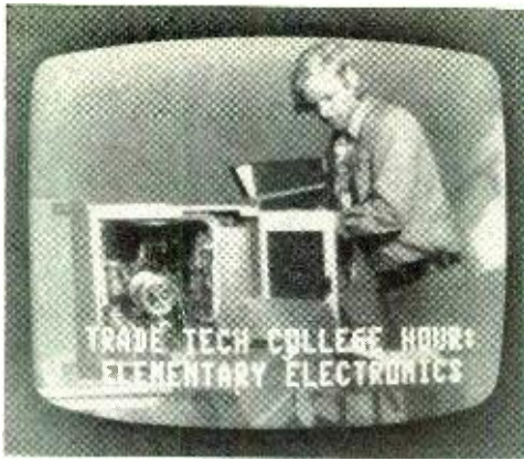
This video display is coded by a special character generator used by the cablecaster.
