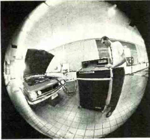
Service technician runs a series of card-programmed performance tests with an Allen automotive diagnostic computer. Results are transmitted by computer printout to owner in lounge.
