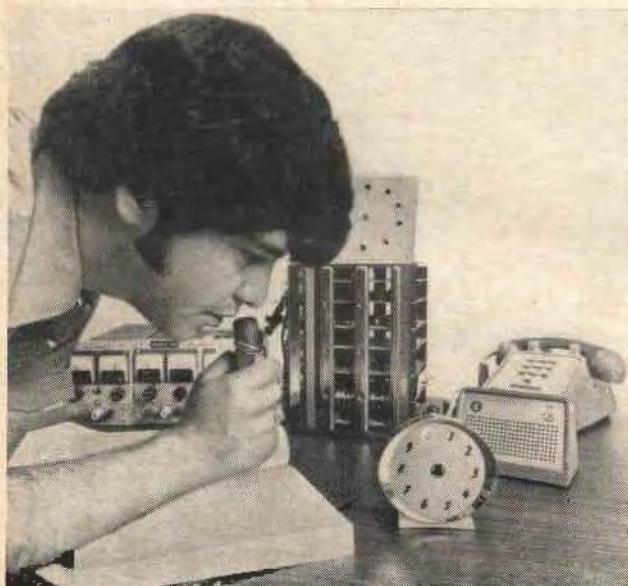
Gerald Soloway, co-developer of a new Bell Labs voice controlled device, "dials" a telephone number simply by speaking into a microphone as numbers appear on the lighted display.
