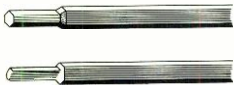
Here are two varieties of plastic adjustment tools for coils: hex (above) and oval.
