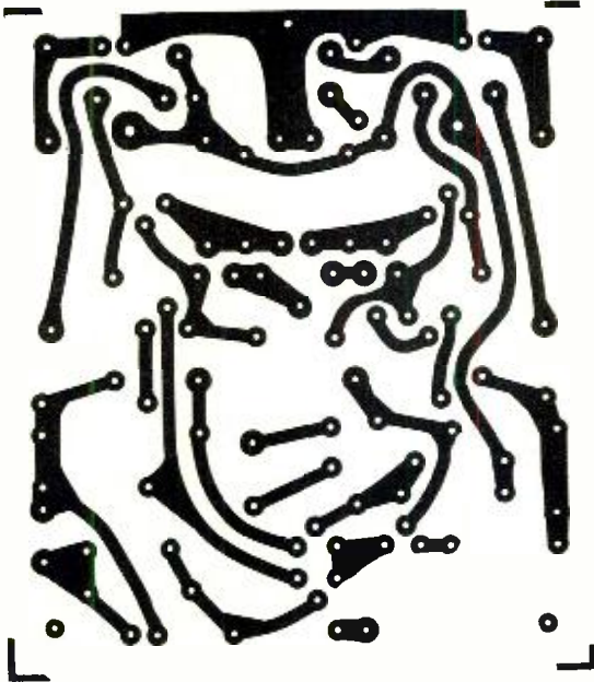
Fig. 5. Actual size etching and drilling guide at left is supplied for those who wish to make their own PC boards. Diagram above shows locations and orientations of components on PC board.
