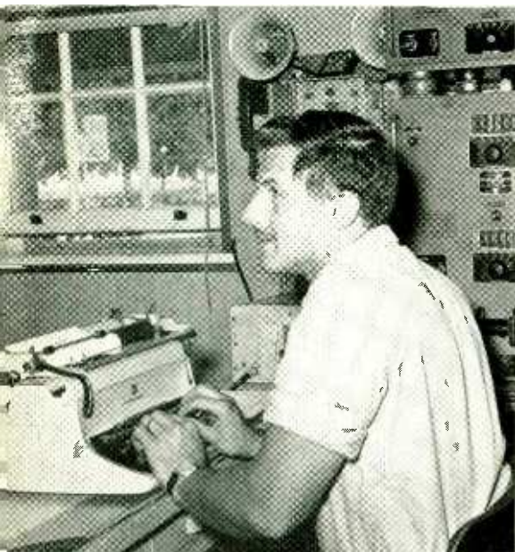
Radioman at Rockaway (N.Y.) USCG Station has harried look as he nears end of 6-hour duty. Receiver at top of panel continually monitors 2182 kHz and has switch knob removed to prevent accidental switching away from distress channel. (Coast Guard Photo)
