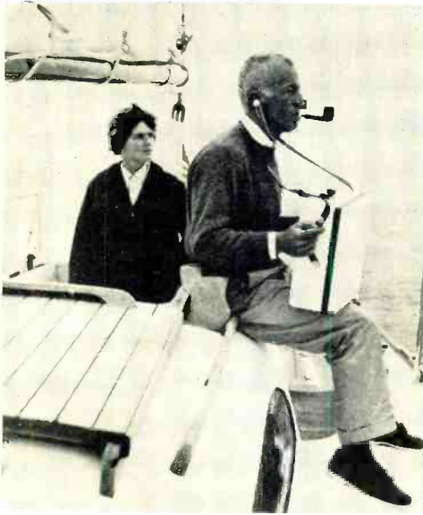
The Whistler is being used here by Roger Merrill of Kimball Products. There is one knob for on/off control and the meter is calibrated in tenths of a mile. Neck strap provides safety in handling.
