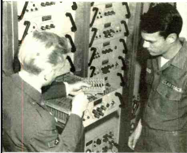
Instructor Sergeant Stephen R. DiStasio of Sacramento, CA, assists Airman Gerald W. Ralston of Grand Fork, ND, in running receiver sensitivity alignment of AN/GRC-169 Collins microwave transceiver (above) in Radio Relay Maintenance course.
