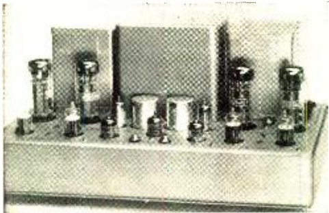
The Audio Research Dual 50 is an all-vacuum-tube power amplifier with impressive figures for output, distortion, frequency response, hum and noise.
