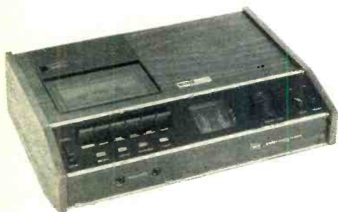
Harman-Kardon's Model CAD5 tape cassette deck is one of the first to have built-in Dolby noise reduction circuits. It can play Dolbyized or not, and Dolby controls can be set for special tapes. Frequency response is improved to beyond 12,500 Hz.
