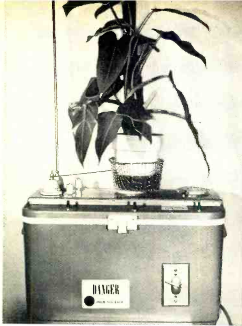
High-voltage electro-culture systems may take the form shown in Fig. 2. The apparatus was designed to investigate the susceptibility of many different plants to stimulation. The equipment generates ozone ( O_3 ) and must be used in well-ventilated areas only.
