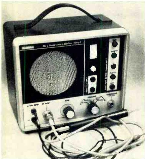
Signal tracer is supplied with two probes—direct for audio tests and an isolated diode rectifier for r-f tests. We dislike fragile tips and tip jacks and plan to substitute sturdy double banana jack and plug at Audio Input on our Signal Tracer.
