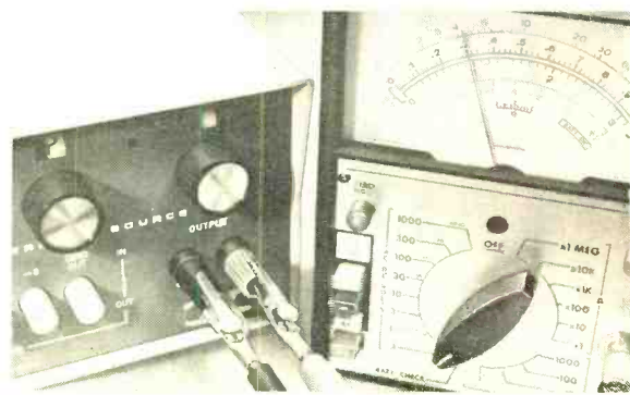
PRECISION LOW VOLTAGE TEST: The 602 passed all tests with flying colors. Using the Heath EU-80-A (see cover photo) and the Lancaster "Mini-DVM", the 602 was well within any possible meter needle parallax error between values of 0.1 and 9.9 volts.
