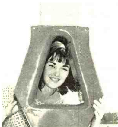
See! It's not uncomfortable at all. The 25-lb elk collar is weatherproof and it is lined. Cross-dipole antenna is on top.
