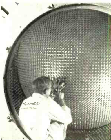
Hughes Aircraft ADAR receiving array consists of a microwave optical system with individual 2°-beamwidth horn feeds. Computer selects beam to track many targets.
