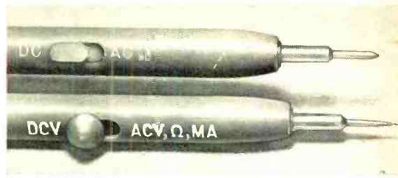
PROBES—NEW and OLD: Triplet made two minor and one major change on the test probe. There is a bigger slide switch button, brighter and bigger lettering and a needle point vs the old tip pin of the 602 probe. Alligator clips are supplied.
