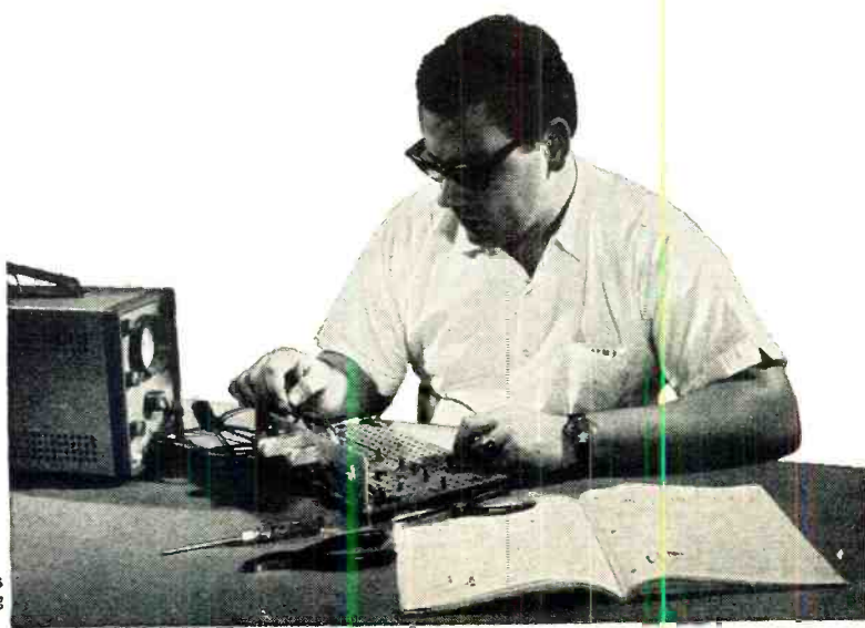
Performing transistor experiments on programmed breadboard—using oscilloscope
