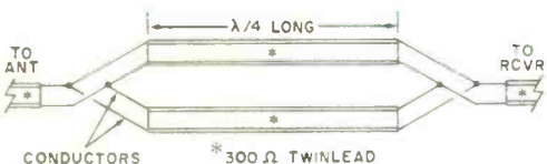
Fig. 1. Transformers are cut to specific lengths for individual channels or for multichannel band.
