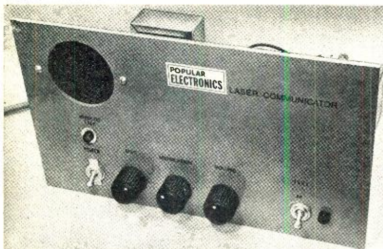
The main chassis for the telescope communicator mounts the relatively heavy power supplies (except for the laser), all controls, and is connected to the telescope electronics via a multi-lead flexible cable. Microphone plugs into the rear.
