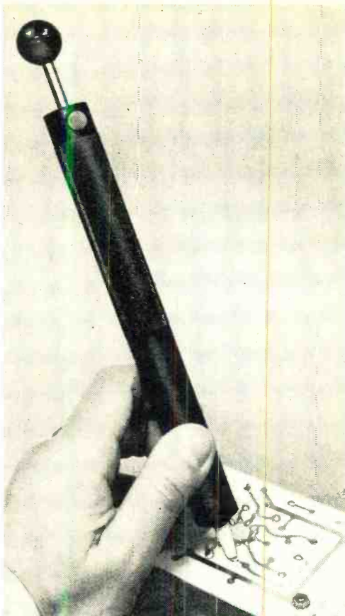
The Continental Products de-soldering tool is operated by depressing the plunger (knob shown at top) to create sucking-pump action. The release for the plunger is the button at top of the barrel and, in this reviewer's opinion, was not in a particularly "handy" location. A redesign to put the release button at bottom of shaft would help.
