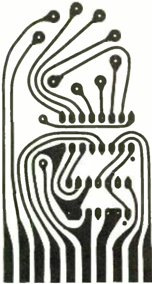
Fig. 2. Actual size printed circuit foil pattern for the readout.
