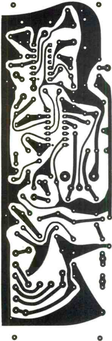
Fig. 2. Actual size printed circuit foil pattern for ultrasonic alarm. Due to circuit complexity, the use of a foil pattern prevents wiring errors.
