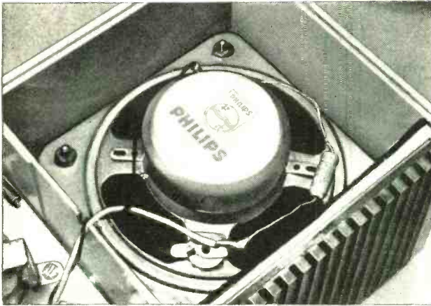
Three views of a non PC board prototype. The photo above shows the use of an IC for each diode bridge, and the larger-sized transformers. The speaker (left) is a 45-ohm type that is mounted on standoffs within the old microphone chamber. The batteries and power switch were contained in the old loudspeaker housing.
