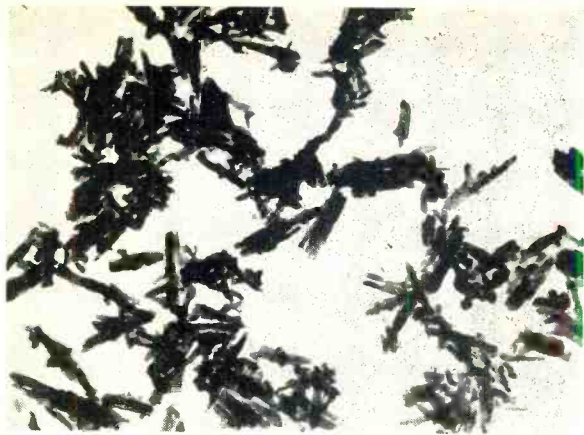
This electron microscope photograph of a piece of audio tape shows the oxide particles; magnification, 60,000 times.
