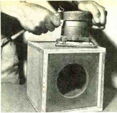
Fig. 6 Power sander is fast way of smoothing surfaces, but you can use wood block and sandpaper.
