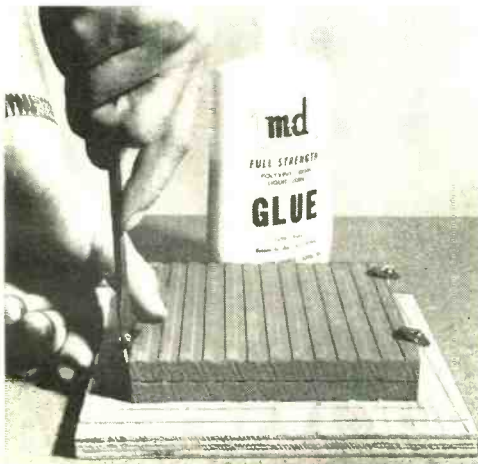
Fig. 2. Bolted down with woodscrews and washers, patio tiles load bottom of enclosure to prevent skidding when the speaker is employed as bookend.
