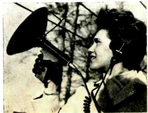
Solid-state sensing "gun" with parabolic reflector can be used to spot punctures in telephone lines.
