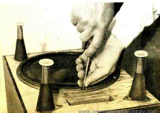
Fig. 2. Because speaker board is fixed by caulking compound, it is necessary to front-mount woofer. Staple or tack grille cloth over speaker cone to protect it against dust and pets.
