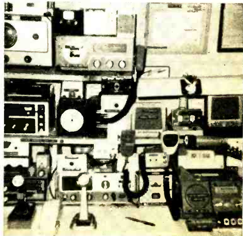
South Suburban REACT (Midlothian, Ill.) serves the Chicago suburban area from this elaborate base station. In addition to monitoring Channel 9, two-way communications are established with local, state, and county sheriff police. Team also monitors fire department communications and U.S. Weather Bureau.
