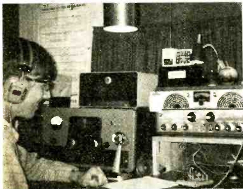
Jim Volstad, WNØTRY, Edina, Minn., really has to crank down the power on his Johnson Valiant transmitter to stay in the 75-watt Novice power limit.
