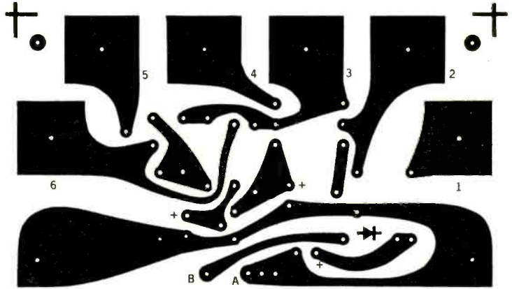
Fig. 2. If you decide to make your own printed circuit board, follow actual-size etching guide shown.
