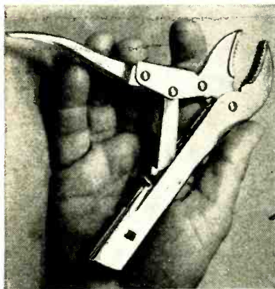
Smaller size LeverWrench will grip anything from thin shim stock to \frac{7}{8} " in diameter. Lower handle flips down and away for quick release. Closing the handle applies pressure automatically to any object held in jaws. Each LeverWrench is supplied in sturdy cowhide leather pouch (see above). Tab on pouch is split for carrying it on your work belt.
