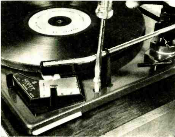
Turntable Holddown. Auto turntable is restrained from bouncing and possibility of motor damage by two "transit screws." The screws may seem to be in backwards—counterclockwise turn to restrain, clockwise to release. Turntable is Garrard 2025TC.
