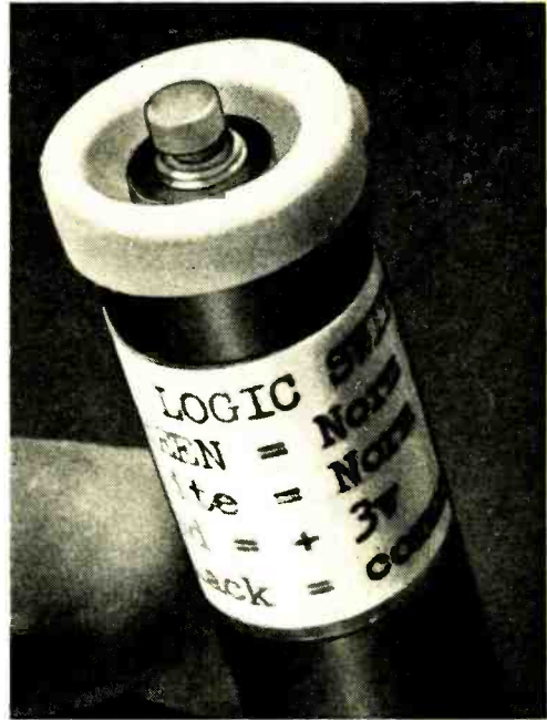
The pushbutton switch fits in a hole drilled in container cover. Like other testers, a typewritten label identifies leads and explains operation.
