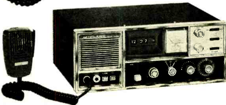
Top-of-the-line from Midland is this Model 13-880 featuring SSB divided 46 channel CB transceiving.
