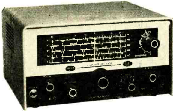
All-solid-state Ameco R-5 receiver has continuous tuning from 0.54 to 54 MHz. May be operated from a.c. line or from an external battery pack. A noise limiter, BFO and band-spread tuning are included.
