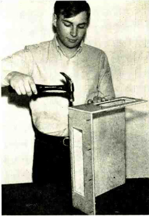
Fig. 2. Sides, bottom, front, assemble with glue and wire brads. Do not allow brads to go into wood at an angle—sides are very thin plywood.
