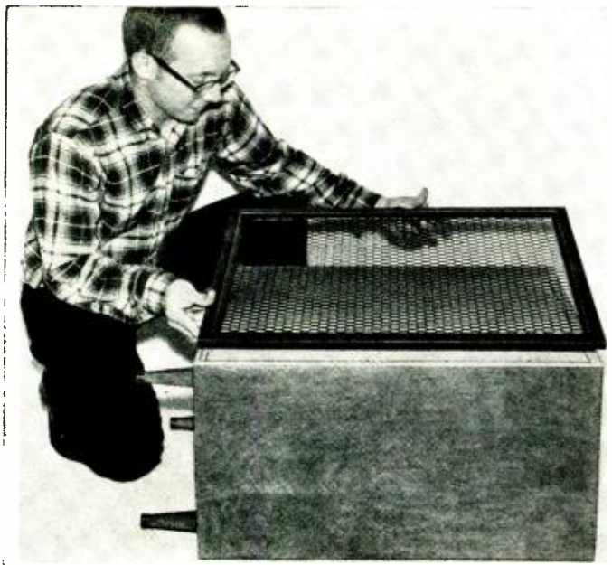
Expanded aluminum grille/picture-frame assembly goes into place only after grille cloth has been tacked onto speaker mounting board. You can use wire brads or ornamental screws to fasten the assembly down.
