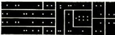
Fig. 2. Actual-size PC board is very small so use care when making it. Unlike conventional boards, this board uses area contact rather than a pattern.
