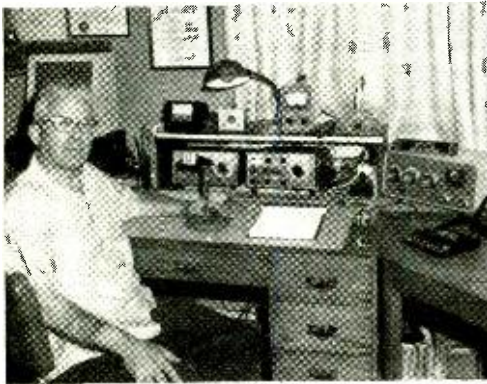
Ray K. Owen, W5UYQ, Oklahoma City, Okla. has his Extra license. His station equipment includes the Drake T4-R4 twins and Heathkit SB-201 linear amplifier. (Photo courtesy Oklahoma City VHF Club.)
