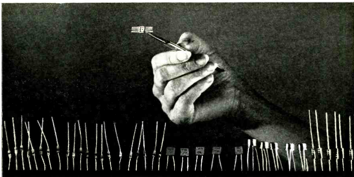
50 functions in a single chip. The functions of 50 separate transistors, diodes, resistors and capacitors can now be performed by the tiny dot in the center of the integrated circuit held by the tweezers.
