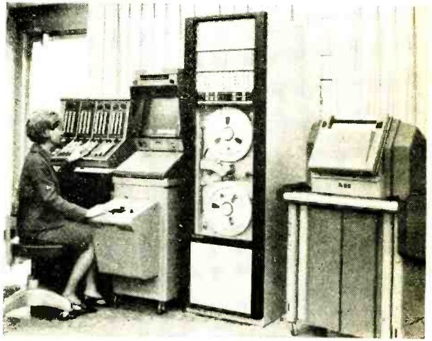
In this fax system, documents retrieved from a microfilm storage are scanned and recorded at high speed for later transmission at low speed on telephone lines. (Photo courtesy of Alden E. & I. R. Co.)
