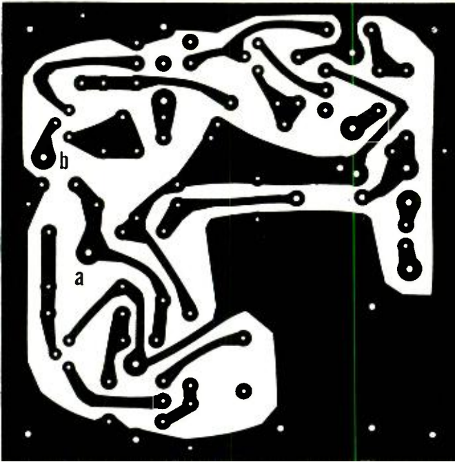
Fig. 2. If you make your own printed circuit board, carefully copy this actual-size etching and drilling guide.
