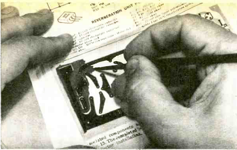
Fig. 2. If you are making your own negative, the first step in preparing a PC board is to place a piece of transparent plastic over the foil pattern. Using opaque paint, fill in areas where copper is to be removed. When it is completed, . . .
