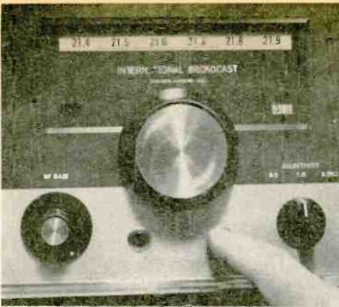
One revolution of SS-1BS dial tunes 10 kHz. Rapid frequency shifting possible with motor drive. Buttons on right goes up frequency, left button down.
