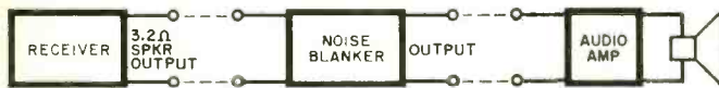
Fig. 3. The noise blanker connects between the receiver loudspeaker output and external audio amplifier.
