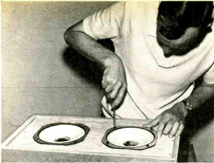
Fig. 4. T-nuts and machine screws are provided to facilitate passive radiator and loudspeaker mounting. Note that the LE8T and PR8 are designed for mounting through the front of the speaker mounting board.
