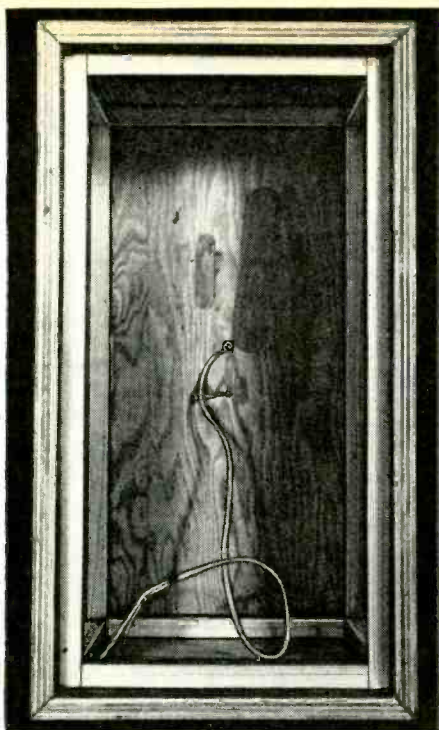
Fig. 3. Two screws, inserted through rear of enclosure, serve as electrical connections.
